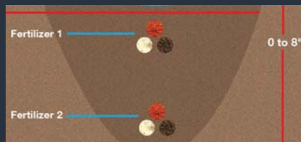
Drop Zone™: allows placement of 2 fertilizer types in 2 independent zones
