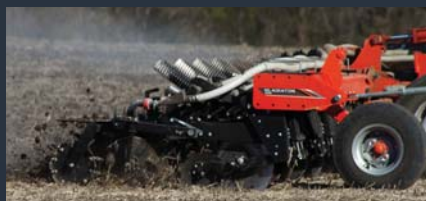
ST-PRO™ row units: create a uniform strip for planting
